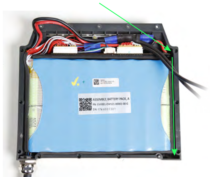
Harness connected. Fit excess wire on the left down into the battery box. Be careful to not damage the circuit board and connectors.
